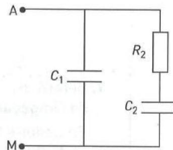
$$Z(j\omega) = \frac{1 + j\tau_2\omega}{j(C_1 + C_2)\omega(1 + j\tau_1\omega)} \quad \text{avec} \quad \tau_1 = R_2 \frac{C_1 C_2}{C_1 + C_2} \quad \text{et} \quad \tau_2 = R_2 C_2.$$
